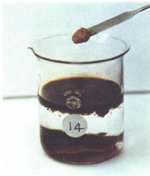
Figure 7 A solidifier that produced a partially floating paste consistency in its solidified byproduct from crude oil.
