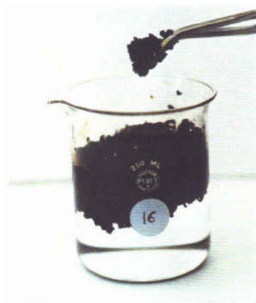
Figure 6 A solidifier that produced a floating non-cohesive consistency in its solidified byproduct from crude oil.
