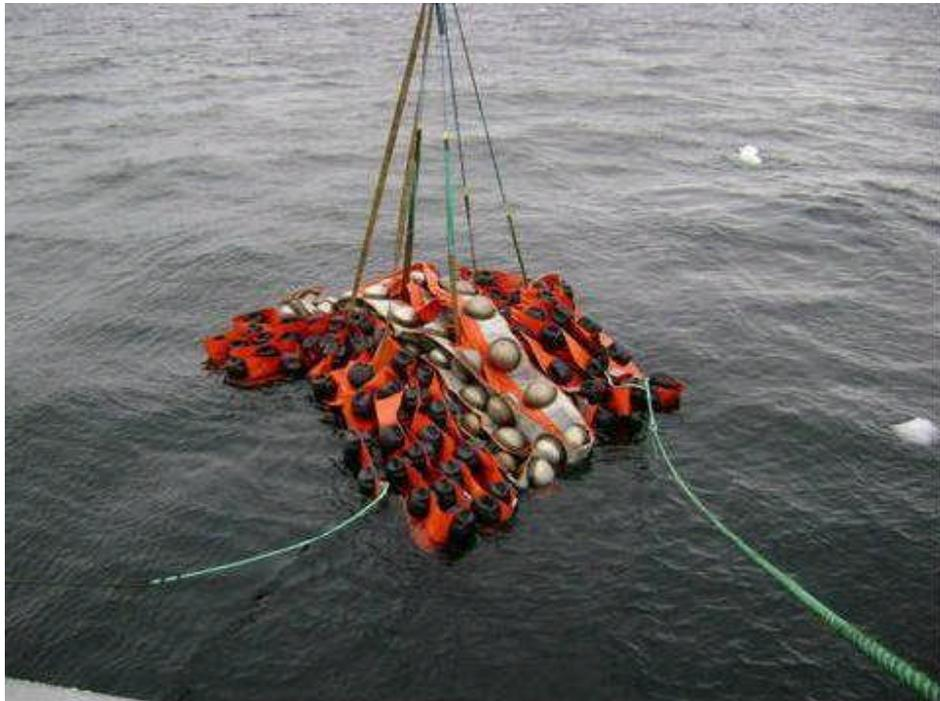
**Figure 2: Deployment of AFTI boom**
